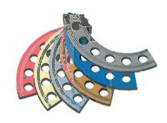
If a threaded rod cannot be inserted into a couple of co-axial ring holes; the conical washers should be used. These allow to incline the rod up to an angle of 15 with respect to the axis of the holes. So doing, rings of different sizes can be assembled, as well as rings with footplates. Besides, the use of conical washers allows to optimize the placement of the clamps for Kirschner wires fixation.
