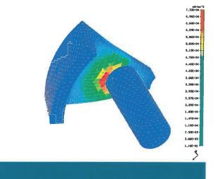
All the components belonging to TFX system have been computer-design by means of finito elements method (FLM), which allows to preliminary compute the stress-and-strain distribution due to the loads application. This allowed the design optimization and the development of devices which, although minimizing weight and volume, are able to safetly factors to take into consideration possible accidental overloads.
