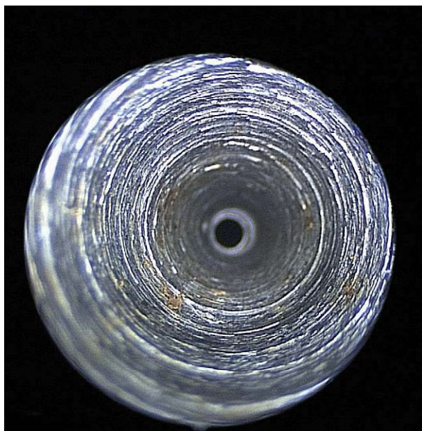
Figure 6. The unpolished interior surface of suction tips allow debris to adhere to the inside.
